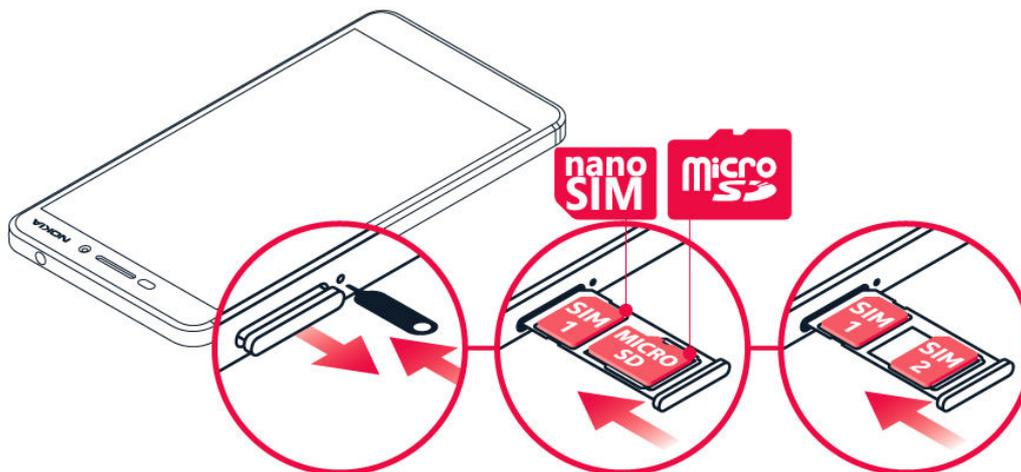
1. To open the SIM card tray, insert the tray opener in the hole next to the tray and push.
